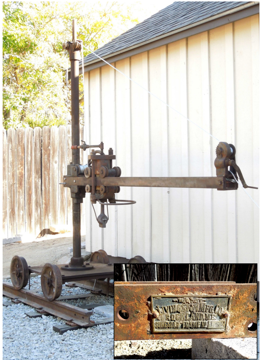
Former quarry operator Roy Ruhkala provided the expertise to restore the 100+ year old pneumatic surfacing machine which had been stored at his home for about 60 years.
