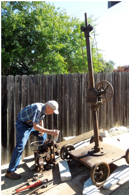
Former quarry operator Roy Ruhkala provided the expertise to restore the 100+ year old pneumatic surfacing machine which had been stored at his home for about 60 years.
